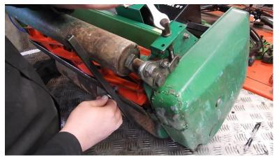
Since grass is cut at the point where the cylinder meets the bottom blade, the height of cut is however far this point is from the ground.
